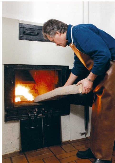
Schlenkerla malt house with beech wood fired kiln
